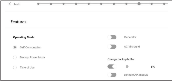
Fig. 158 Self-Consumption mode with AC Microgrid and Backup Buffer
