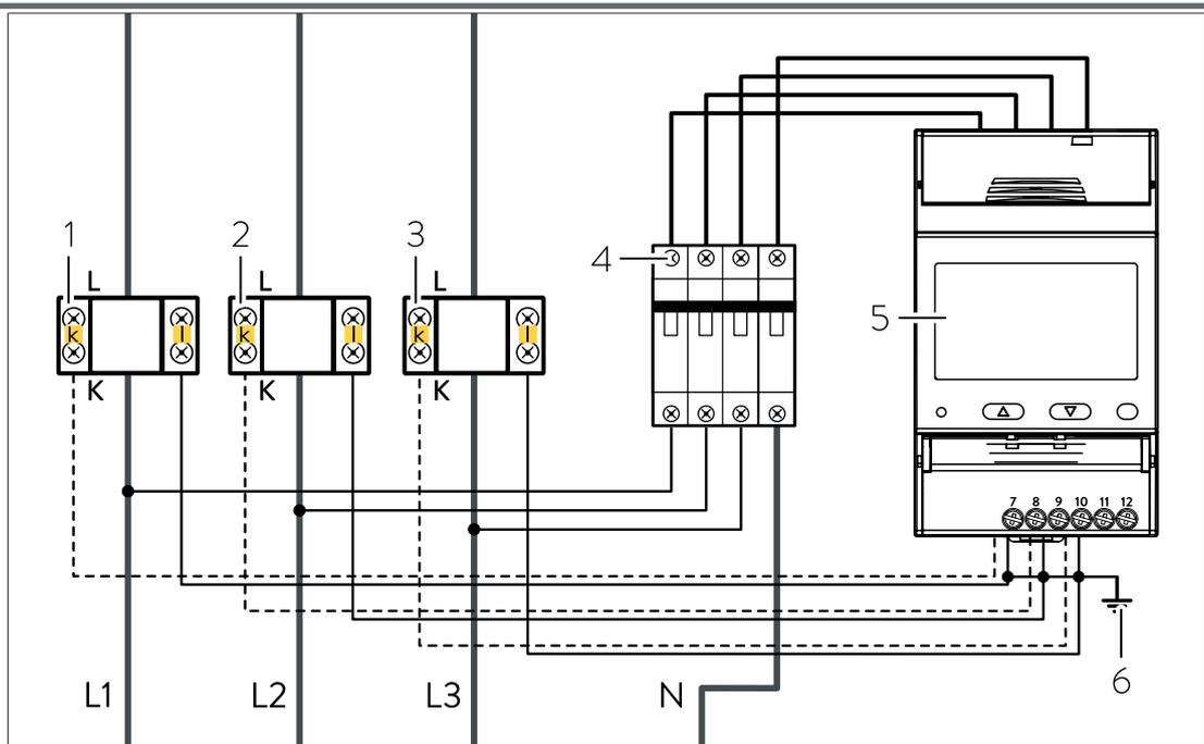
Illustration 20: Connection for measuring a measurement point with the EM530 power meter and current transformers
