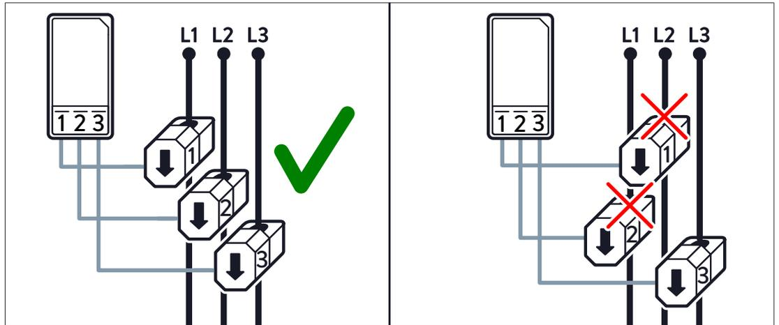
Illustration 5: Connecting the clamp-on current transformers - incorrect (right) and correct (left)
