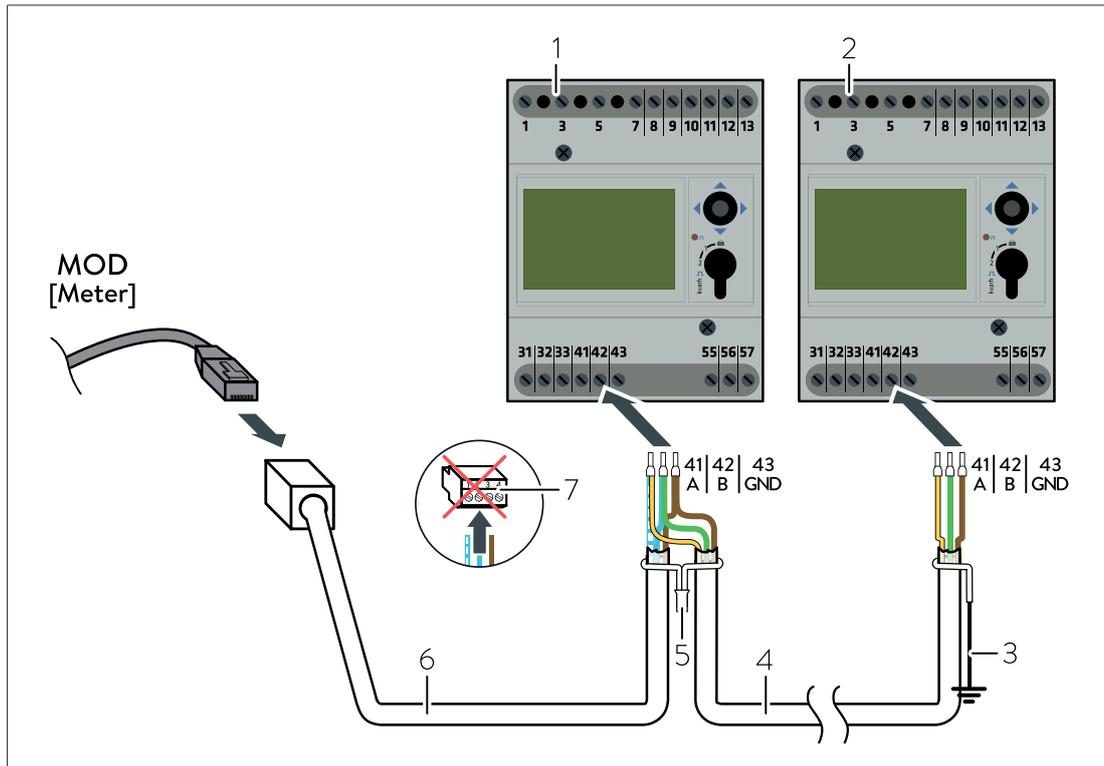
Illustration 22: Connecting the communication line when two WM10 power meters are used
