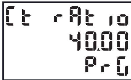
Illustration 28: Ct rAtio screen, set to transformer ratio 40
