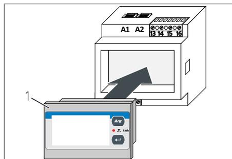
Illustration 9: Inserting the touch display
