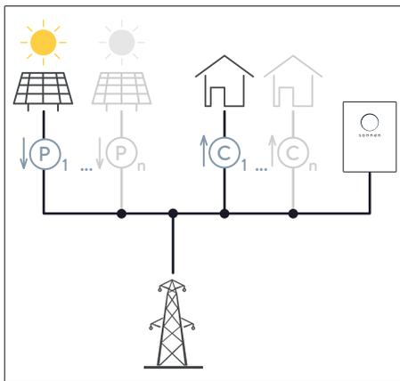
In this concept the production is measured at point P1 and the consumption is measured at point C1.
