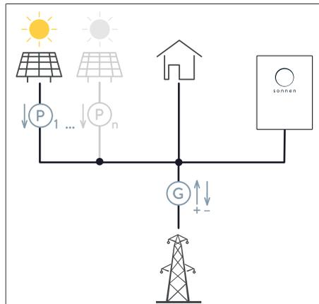
In this measurement concept, the power consumed is measured at point P1. Further measurement points (P2 to Pn) can be integrated into the system. In this case the total production results from the sums of the individual measured values.
