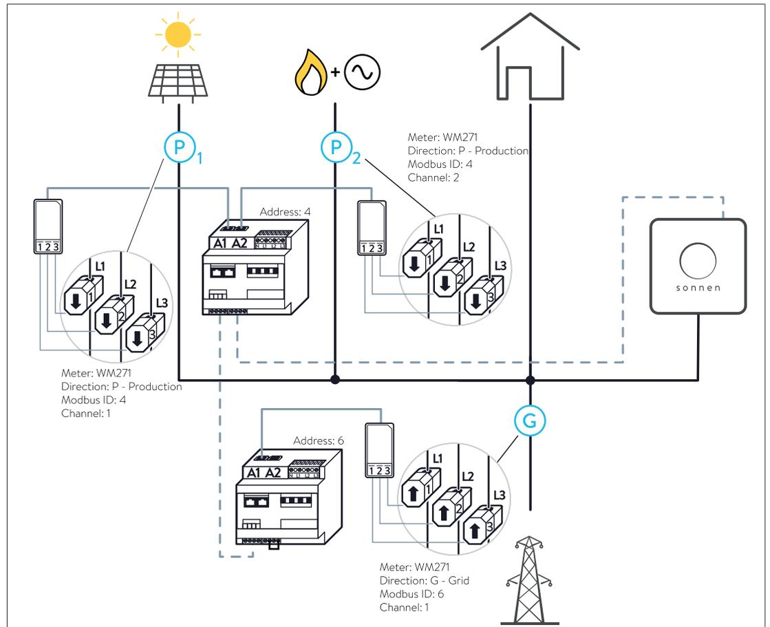
Illustration 41: Example for the implementation of the GP measurement concept - The circles show the connection of the CTs at the three measurement points
