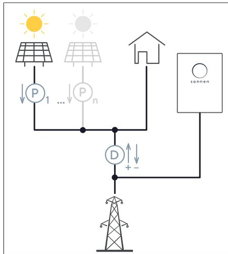
In this measurement concept, the power consumed is measured at point P1.
