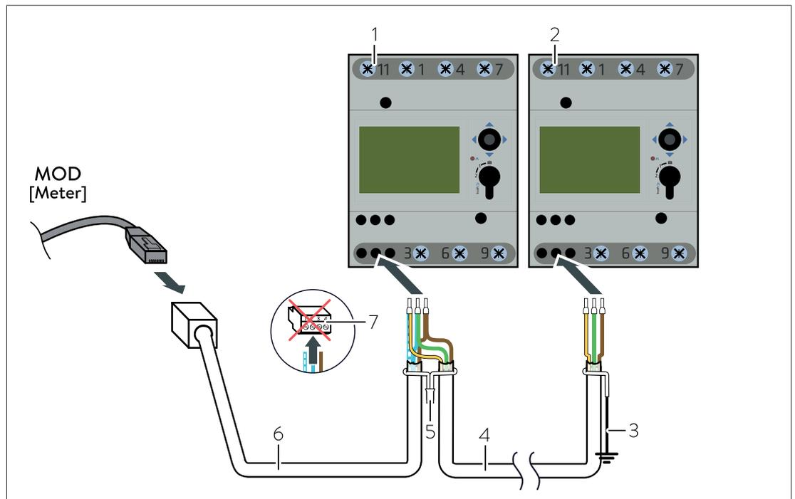
Illustration 23: Connecting the communication line when two WM63-M power meters are used
