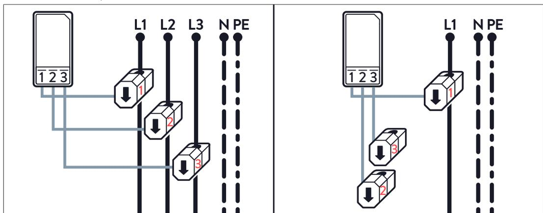
Illustration 4: Connecting the clamp-on current transformers for three-phase and single-phase measurement
