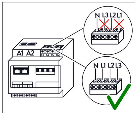
Illustration 6: Connection to the voltage terminal strip - incorrect (top) and correct (bottom)
