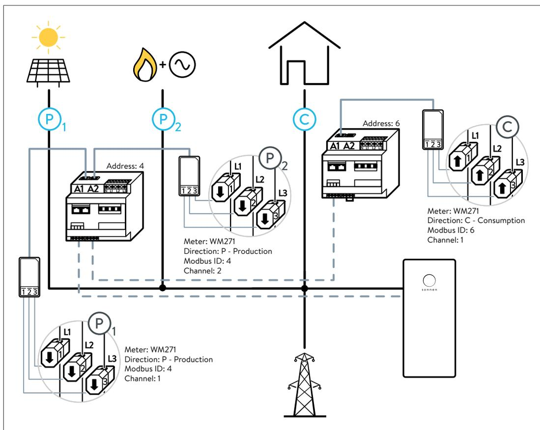
Illustration 40: Example for the implementation of the CP measurement concept - The circles show the connection of the clamp-on current transformers at the three measuring points
