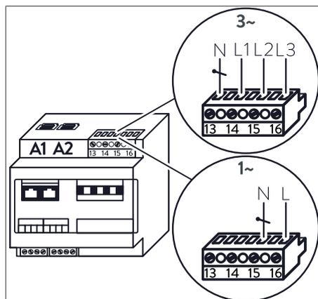
Illustration 3: Connection to the voltage measurement terminal strip at single-phase and three-phase mains
