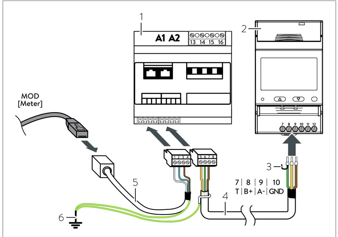
Illustration 36: Example connection of the communication lines for the WM271 and EM530
