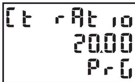
Illustration 29: Ct rAtio screen, set to transformer ratio 20
