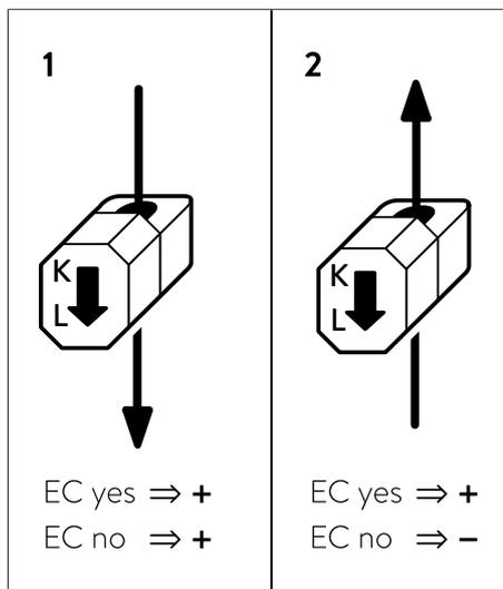
Illustration 19: Case 1 (left): the energy flow in the conductor s from K to L | Case 2 (right): the energy flow in the conductor is from L to K
